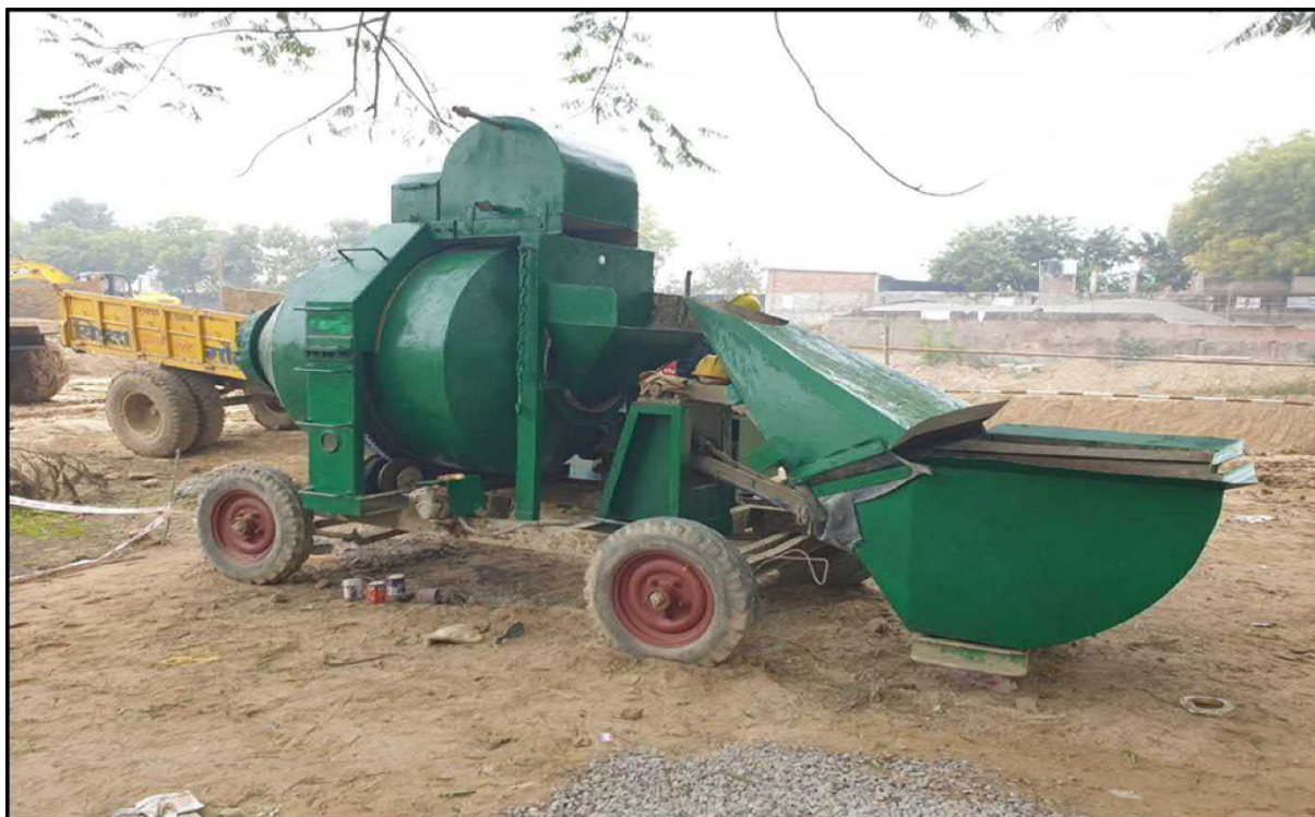
Mixture Machine RM-800 installed at site
